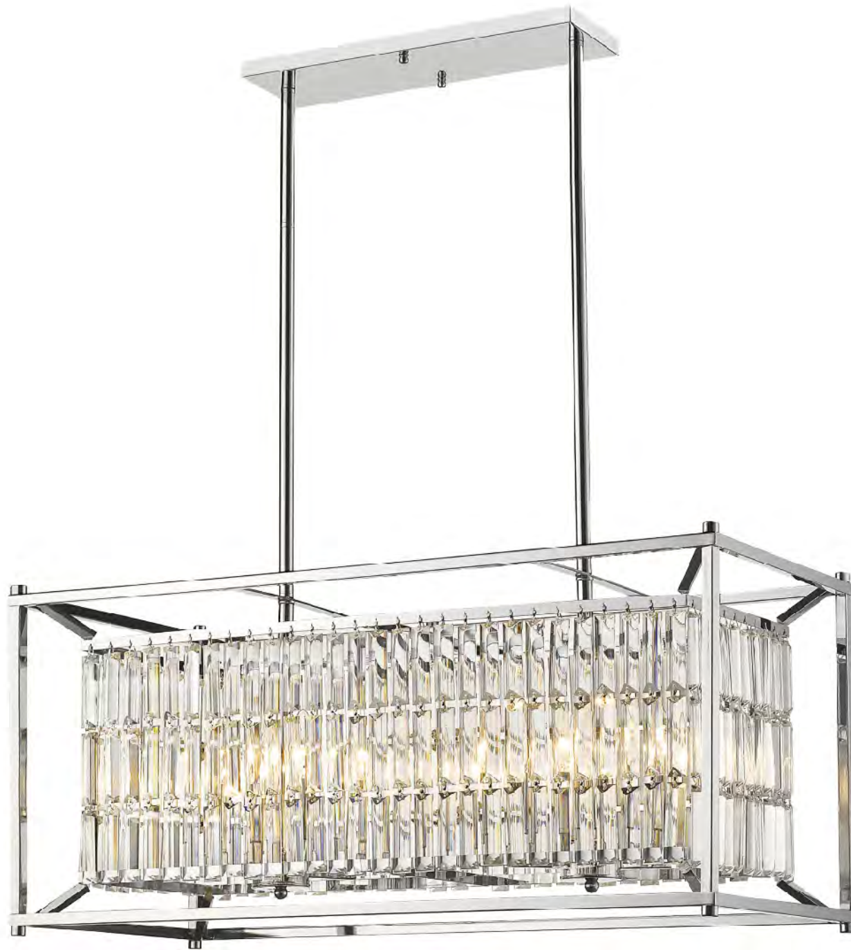
YS6222-8P SIZE:31.5"L×13.75"W×13.75"H LAMP:8/60W/E12 YS6222-8P-GD (OUTSIDE FRAME CHROME& INSIDE SOCKET AND PARTS GOLD)
